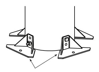
One or two pairs of pole bearing plates can be used. Note how each pair mounts with one bolt through upper or lower locating hole.
